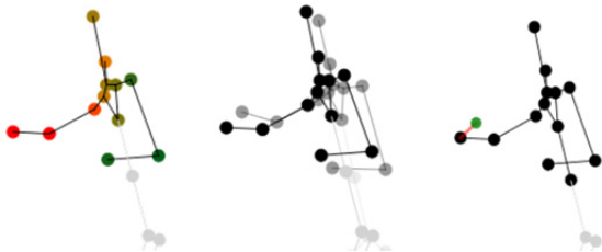
Figure 6: Exemplary skeleton-based distance error visualizations (left: colored joint overlay, center: overlay of template and comparison skeleton, right: static result of animated joint moving to its correct position).
